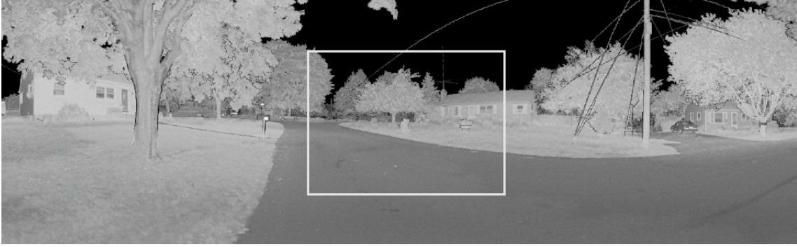
Figure 1 Panoramic projection of the 3D data of a range-image, brightness encodes the intensity of the reflected laser beam, i.e. white: high intensity, black: vanishing intensity.
